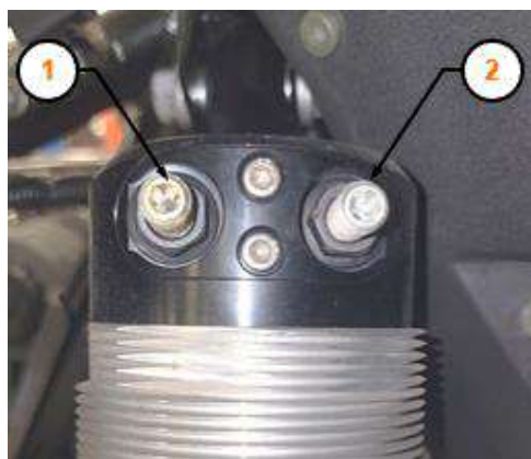
1: Compression Adjuster (LEFT) 2: Rebound Adjuster (RIGHT)
