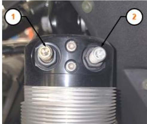
1: Compression Adjuster (LEFT) 2: Rebound Adjuster (RIGHT)
