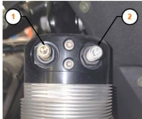
1: Compression Adjuster (LEFT) 2: Rebound Adjuster (RIGHT)
