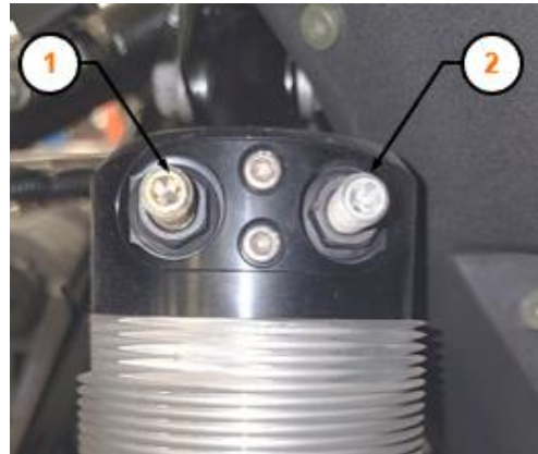
1: Compression Adjuster (LEFT) 2: Rebound Adjuster (RIGHT)
