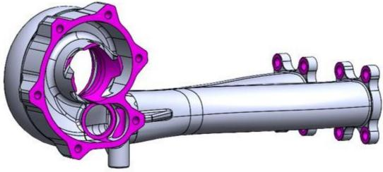
A one piece manifold/turbine housing is the best solution because it eliminates all failure points. We have experienced failures at every other type of connection attempted (bolts, v-band, expansion joints)
