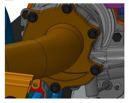
Because the wastegate flow in re-integrated into the main exhaust flow, there is no need for a complex housing shape to trey and capture the wastegate air as well
