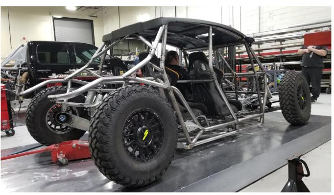
At full bump there is ~3" of clearance between the chassis and ground.
