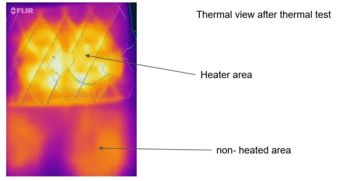
PCT self regulating material heats up quickly (~1 min) to operating temp 95-105 F and maintains temperature.
