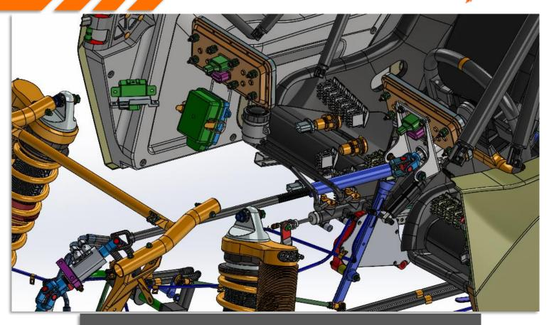
An adjustable floating column also prevents binding from U-joints.
