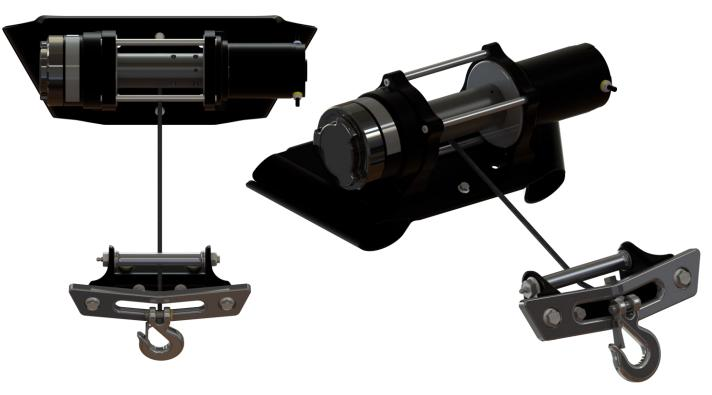
The winch is rated for 4500LBS Bolt in installation. (Requires Grill Modification)
