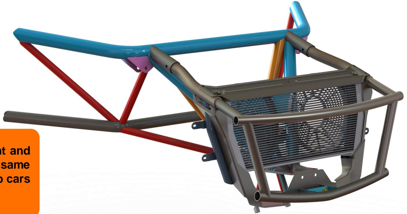
**Front bumper mount and core support is the same on the enclosed cab cars (with radiator)**
