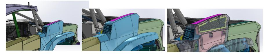
We have More than doubled the Suraface area of the number plate intake for engine and CVT cooling
