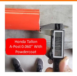
Cheap, thin walled tube 2" OD 0.049" - 0.078" Wall
