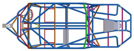
New Revisions to Lower Frame Structure for increased Rigidity.
